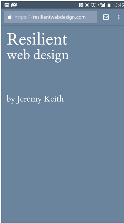
FIG 9.1: The interface of the Chrome browser on Android takes on the theme_color specified in the Web App Manifest for the web book Resilient Web Design ( http://bkaprt.com/go/09-03/ ).
